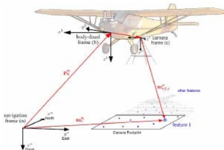
Figure A.14 Relationships between UAV position and orientation, feature (cactus) position and observation by the on-board camera, all used for mapping the location of observed cacti
