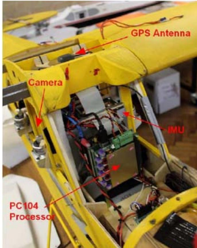
Figure A.2 Internal view of the J3 Cub UAV system, showing payload box incorporating the inertial measuring unit, the GPS receiver and antenna, the vision-stack processor and the camera system
