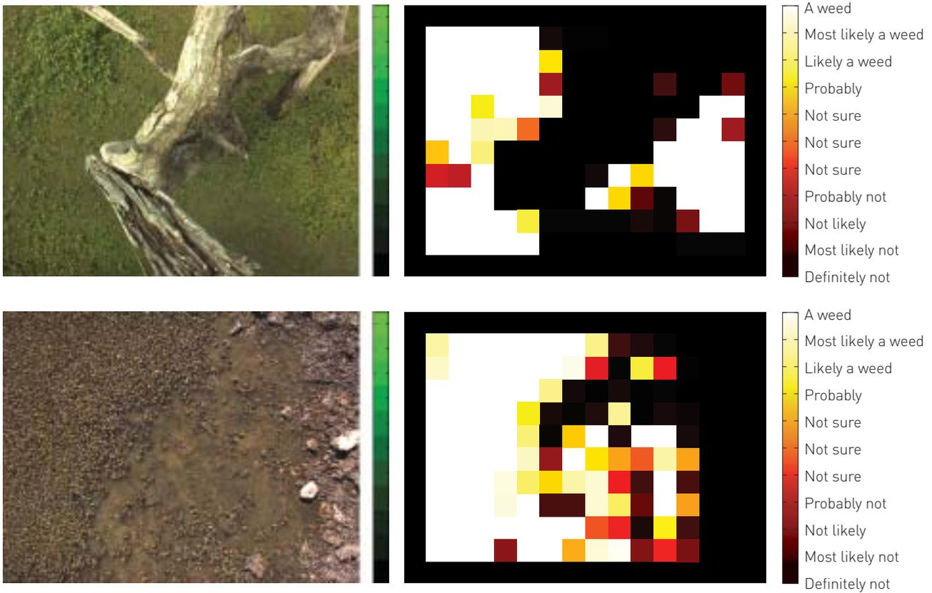
**Figure 3.** The top images represent the classification results of alligator weed, and the bottom that of sprayed salvinia. The images in the left hand column are those directly from the imaging system, and that in the right hand column are the output of the learnt classification model.
