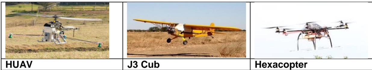
**Figure 2.** ACFR aerial robotic platforms used in pest detections
